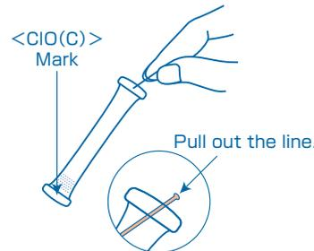
② Remove the colored line at the top of the tube to clear the aperture.
