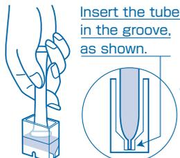
Insert the tube in the groove, as shown.
