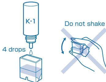
① Fill the Cell (PACKTEST Square Cup) up to the line (1.5mL) with sample. Add 4 drops (about 0.25mL) of K-1 Reagent.
