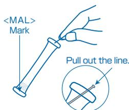
② Remove the colored line at the top of the tube to clear the aperture.
