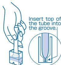
④ Immerse the aperture of the tube into the Cell, pressing it against the bottom, and release to take all the sample from the Cell into the tube. Shake the tube lightly for 15 times and dissolve reagent completely.
